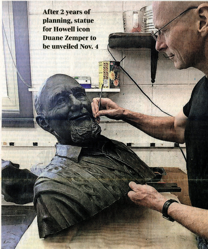
The bust portion of the Duane Zemper statue was combed by Colin Poole, of Santa Fe, New Mexico. He and his wife Kristine were commissioned to create the statue. "We use fine stainless steel tools to remove seam lines left on the wax from the mold, repair any defects (like bubbles) and refine details," Poole said. COURTESY OF COLIN POOLE
